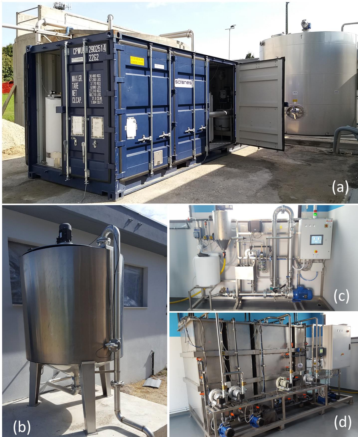
Figure 2 (a) Salsnes Filter SF1000 for the sieving of wastewater; (b) fermentation unit for the production of VFAs; (c) ceramic membrane for the solid/liquid separation and crystallizer for P-salts production; (d) Units in SBRs-modules for nitrification, PHA storing biomass selection and PHA accumulation.
