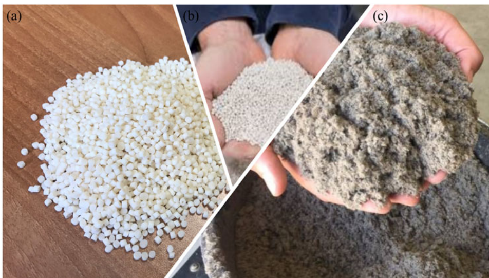
Figure 1. Examples of the recovered products in the context of SMART-Plant Project (a) Recovered PHA from SMARTech2b in Manresa WWTP, Spain (b) Recovered struvite from SMARTech5 in Carbonera WWTP, Italy (c) Recovered cellulosic sludge from Geestmerambacht WWTP, Netherlands.
